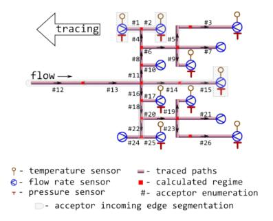
In latter case no more than two nodes must be equipped with pressure and temperature sensors whereas for other nodes only flow rate sensors must be installed.
