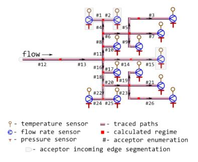
As it may be seen from the figure there is a particularity in topology of the provided directed graph: each node has only single ancestor. Hence one of isomorphic representation of such directed graph is a data.frame in which each row describes a node along with its incoming edge and each column contains an attribute value for that node or an attribute value for its incoming edge.
