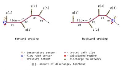
They make additional check for consistency of inlet and outlet values for subsequent pipe segments. Discrepancy of appropriate elevations cannot be more than elev\_tol.
