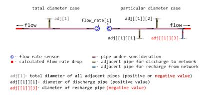
Usually, there are no additional sensors that could measure flow rate in each flow fork. In that case they only may operate with geometric factors, i.e. assuming that flow rate is proportional to square of pipe diameter.
