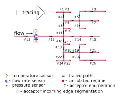
Tracing starts from sensor-equipped root node and goes forward, i.e along the flow direction. Function traceline serves under the hood for tracing identified linear segments from root node to every terminal node. Hence they only need root node to be equipped with sensors. Sensors at other nodes are redundant in forward tracing, since the tracing algorithm by no means consider them for tracing.
