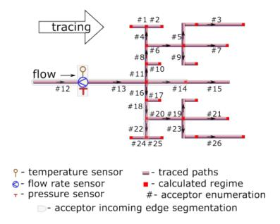
Tracing starts from sensor-equipped root node and goes forward, i.e along the flow direction. Function m325traceline serves under the hood for tracing identified linear segments from root node to every terminal node. Hence they only need root node to be equipped with sensors. Sensors at other nodes are redundant in forward tracing, since the tracing algorithm by no means consider them for tracing.
